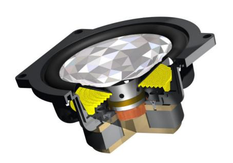
Due to the high rigidity of the aluminium membrane, it is now possible to attach the solenoid not only to the cone neck but also directly to the aluminium membrane. This significantly extends the cone's bandwidth right across the frequency range giving a noticeably more even & continuous frequency response.
